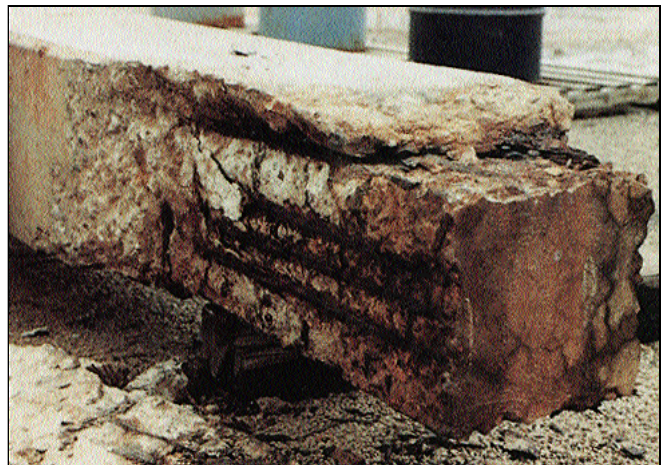
Figure 5. The nonconductive material used to repair this beam (top) accelerated the corrosion of reinforcing steel, which led to premature repair failure (bottom).
