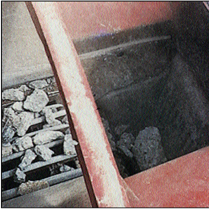
Figure 4. Screens directly below this primary crusher separate fines from the crusher output.
