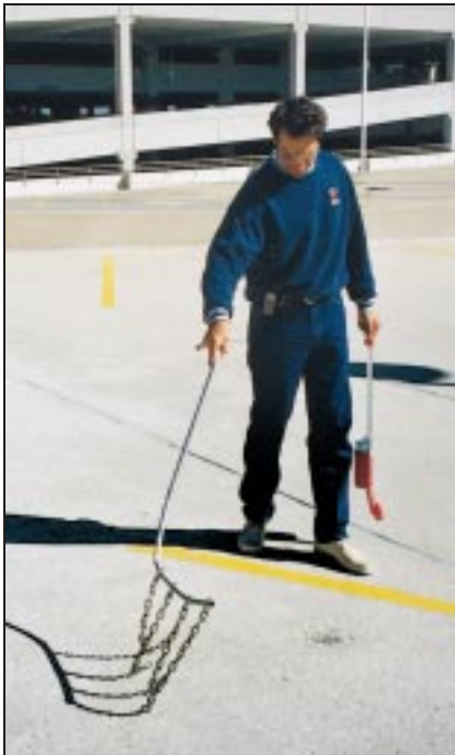
Figure 1. Chain dragging is a simple yet effective way to locate delaminations in reinforced concrete.
