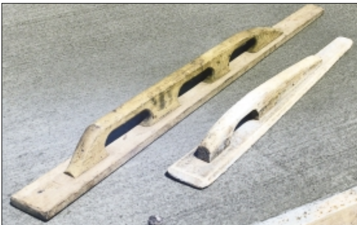
Above: Darbies serve the same purpose as bull floats except they are used on smaller areas and are moved across the concrete surface in a sawing arc instead of a back-and-forth motion. Right: If you prefer to stand while edging, use a walking edger that attaches to a long handle. One type of handle bracket allows you to flip-flop the handle to either side of the edger. Another type (shown here) locks the handle in a set position.
