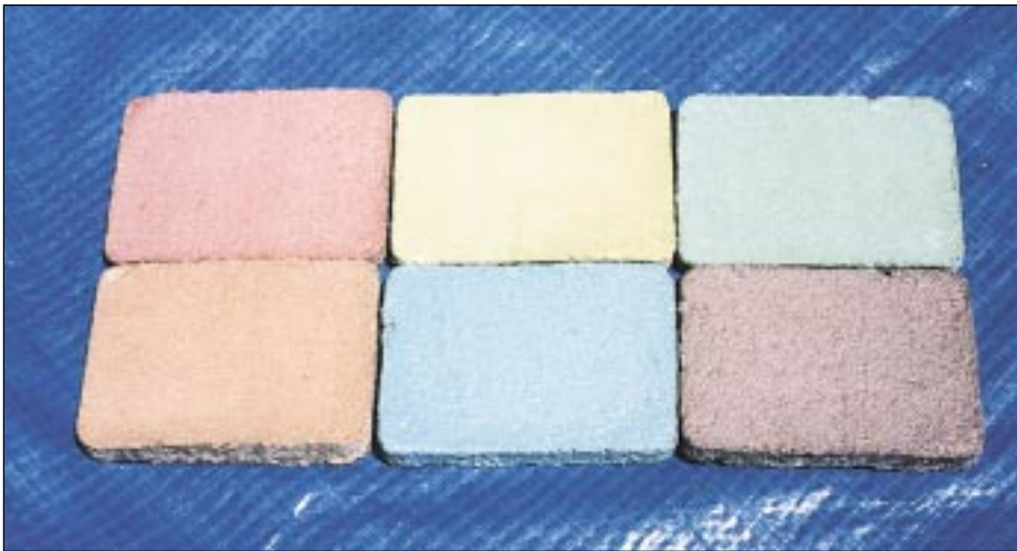
Left: Flowable fill is available in the colors shown on the samples. Below, left: Measuring flowable fill sample diameter to estimate flowability of material. Below, right: Test cylinders are filled with green flowable fill. Cylinders have drainage holes to simulate field conditions.
