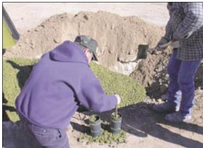
Left: Flowable fill is available in the colors shown on the samples. Below, left: Measuring flowable fill sample diameter to estimate flowability of material. Below, right: Test cylinders are filled with green flowable fill. Cylinders have drainage holes to simulate field conditions.
