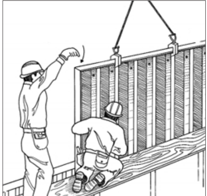
Two simple, basic safety rules were not followed: First, never work under a suspended load. Second, a crane operator never leaves the controls with a load hanging.
