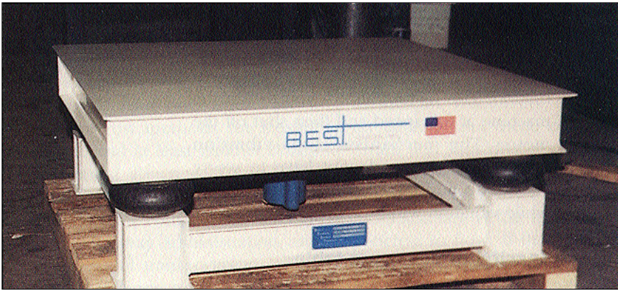
The air-mount isolators on this flat-top table keep vibration confined to the table top and mold.
