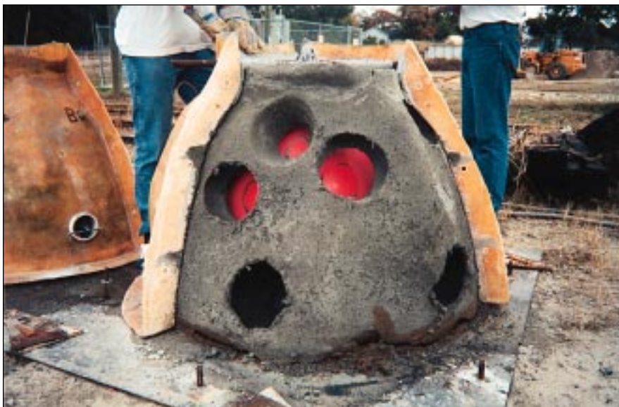
Demolding of a Reef Ball reveals its Swiss-cheese-like holes and internal inflated balloon.
